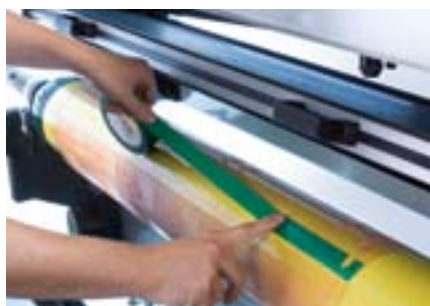
Sealing the edges.
