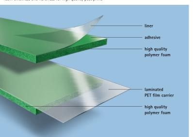
Expertise in every layer: the double-sided flexible reinforcement in foam mounting tapes made by Lohmann ensures continuous production of top quality print results.
